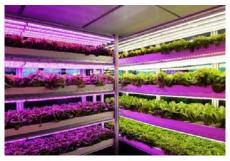
Due to the stacking of plant layers the plants grow completely under artificial light without any daylight at all. This is also referred to as sole-source lighting. This gives complete control over the timing, amount and spectral composition but also requires a complete light content. If people work under these lighting conditions a white light impression is necessary to enable the workers to assess the quality of the plants.
